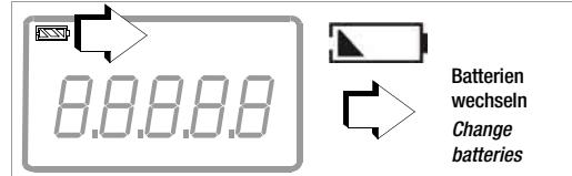
**Batterietausch – Battery Replacement**
